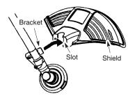
2. Secure shield to bracket with bolt.
